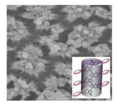
Nanorod arrays of functionalized poly(3,4-ethylenedioxythiophene) (PEDOT) are assembled by using an anodic aluminum oxide template directly fabricated on gold-coated silicon wafers. These nanorod arrays are promising for organic electronic and biomedical applications. This approach allows a platform to understand the molecular and nanostructural effect on the surface wettability of these materials.
