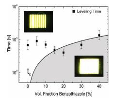
The interplay between surface tension, viscosity, and drying time of organic semiconducting inks is taken into account to fabricate homogeneous active layers for organic light-emitting diodes (OLEDs) by gravure printing. The optimal formulation of the ink is identified when its properties allow a film leveling time shorter that the critical "freezing" time.
