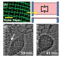
A methodology to develop suspended structures with tunable Poisson's ratios is reported. Two-photon polymerization is used to fabricate suspended web structures with a negative Poisson's ratio (NPR), based on analytical models. This technique could be used to investigate effects of altering the Poisson's ratio of several photocurable biomaterials on a variety of cellular aspects including morphology, gene expression, and migration using different cell types.
