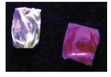
Electrospun nonwovens with chameleontype surface properties are obtained by green electrospinning of acrylate dispersions with ionic moieties followed by photo cross-linking. The resulting chameleon nonwovens can be coated by layerby-layer deposition with a large variety of different functional materials including dyes, antibacterial compounds, silver, and gold nanoparticles.
